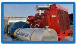
Model: - Jet stream 4215D, Max power is 350hp, Trailer mounted UNx water blast system 15k.
